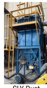
SLY Dust Collector/ Bag House
